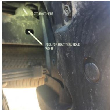
Figure 7 Left Center Bolt Lube Location
