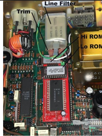
Finished installation in Fluke 8842A
