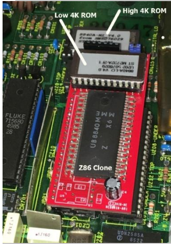
Finished installation in Fluke 8840A
